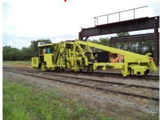
TM Track's **6700 Hybrid** process takes a used 6700 tamper down to the sandblasted frame and "Re-Manufactures" it with all systems and components refurbished, rebuilt or replaced with new parts. The **6700 Hybrid** delivers exceptional "mainline" Switch/ Production Tamper performance in a modern, operator-friendly environment.
