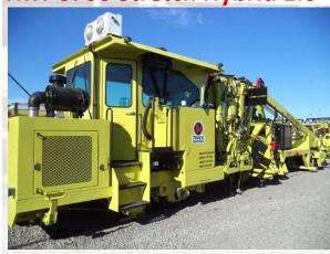
TM Track's **6700 Stretch Hybrid** process turns little ones into big ones. A legacy "Small Cab" 6700 is "Stretched" to the size of a modern "Big Cab" 6700, and "Re-Manufactured" with all systems and components refurbished, rebuilt or replaced with new parts.
