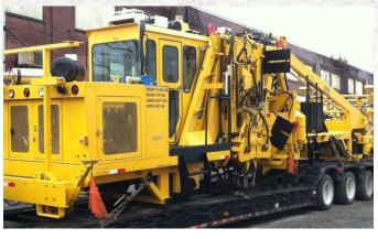
TM Track's **6700** Reman Tamper delivers exceptional Switch/Production Tamper performance from either a legacy "Small Cab" or "Big Cab" 6700 at the end of its original service life. A legacy 6700 is "Re-Manufactured" from the sandblasted frame up, with all systems and components refurbished, rebuilt or replaced with new parts.
